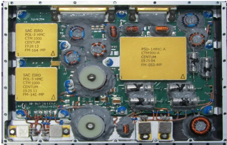
PCPU for C-band TR Module 60W EPC for X-band TR modules for active antenna
