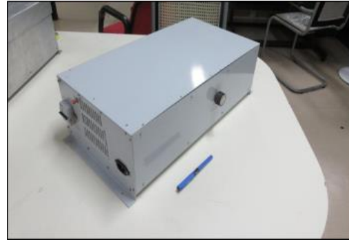
Miniaturized device prototype developed by SAC/ISRO for corona virus fragmentation using microwave radiation.
