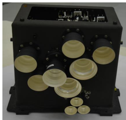
Ka-band Multiple Beam Antenna with different size beams ( communication cum RF Tracking Feed )
