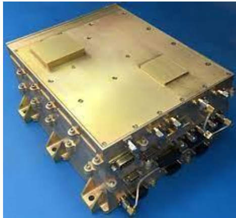
Multi-level stacked package example
