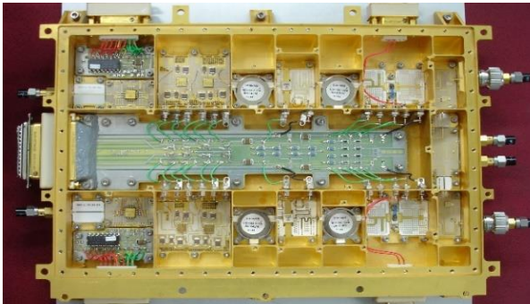
GaN based Dual Pol Pulsed Transmitter for Chandrayan-II
