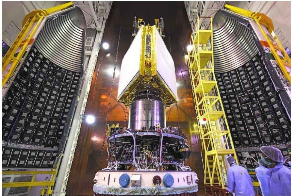
EOS-4 Satellite inside Payload Adapter at SDSC SHAR Centre
