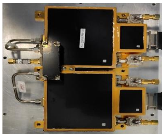
Ku-band 4-channel Transmit Module
