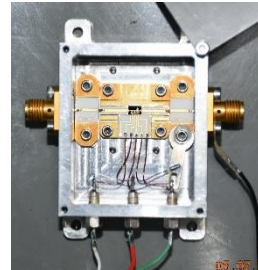
7 to 12.5 GHz Low Noise Amplifier MMIC
